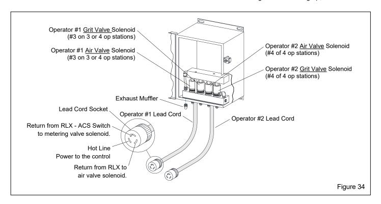
Figure 34. The slot to the left (counter-clockwise of the angled slot) is the hot line, which carries the power from the panel to the RLX control handle.
