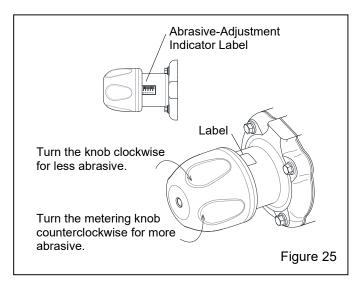
**5.1.3** Optimum abrasive flow depends on the type and size of abrasive and blasting pressure, and can best be determined by experience. Use as little abrasive as possible while maintaining the maximum cleaning rate. The air-abrasive mixture should be mainly air. As a rule,
