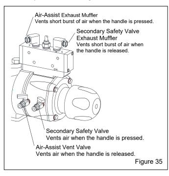
**8.5.3** Release the control handle lever. A short burst of air should come from (Port 5) the secondary safety valve exhaust muffler, and air should now come from the air-assist vent valve.
