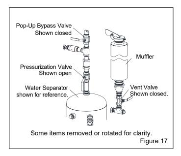
**4.3.2 Depressurizing the abrasive chamber:** Close the pressurization valve and open the exhaust valve. The pop-up valve automatically drops when air is expelled from the chamber and pressure equalizes.
