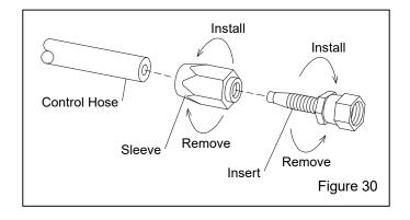
**7.6.5** Push the end of the insert into the sleeve and turn it clockwise to tighten until the insert hex is against the sleeve.
