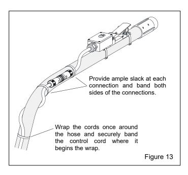
NOTE: Wrapping the cord provides slack; if the cord is not wrapped and securely banded as described, excessive strain will cause the wires to pull out of the connectors or electric switch when the hose is bent or pulled.
