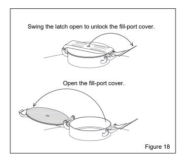
**4.5.5** It is not necessary to close the cover when the chamber is full; close the cover when required by weather or at the end of the blasting shift to prevent moisture and foreign material from entering the chamber.
