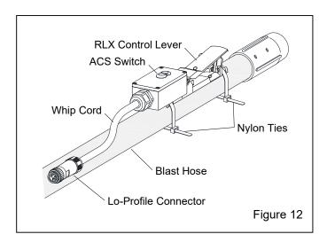
**2.5.2.6** Working from the control handle back, band the cord to the blast hose every 4 to 6 feet. Also, band the cord on both sides of each electrical connection.
